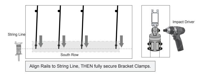
Install the Rails along the remaining rows of Bracket Clamps, adjusting the Post Mount heights as needed to achieve the slope specified in the project plan set. Fully secure ALL Bracket Clamp and Post Mount fasteners.
