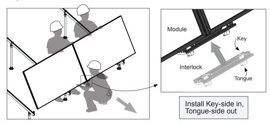
(E) Align the Interlock so that the edges of the modules fall on the appropriate timing marks.
