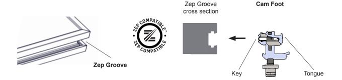
In ZS Ramp, the Key side of the Cam Foot inserts into the Zep Groove, securing the module in place. The locking process is auto-bonding.
