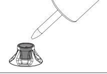
Cover the surface of the inside of the base foot for a complete, waterproof seal.
