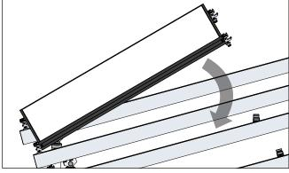
(E) Insert the Cam Feet into their respective Rail channels and use the Flat Tool to secure them 90 degrees clockwise.
