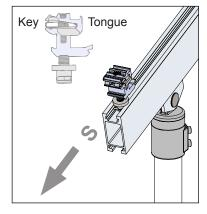
Keep the Offset Flat Tool parallel to surface to avoid gouging the Rail.
