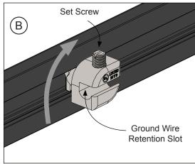
**Installation:** Insert a Ground Zep into the Zep Groove with the label facing out and set screw pointing left. Use the Zep Tool (or Flat Tool) to turn the Ground Zep 90 degrees clockwise so that the set screw is pointing up.
