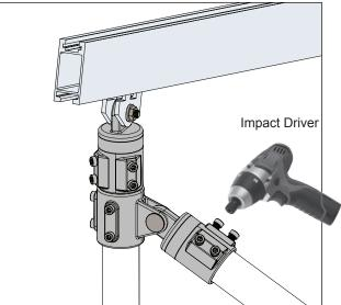
FIRST, secure the Tube Head onto the Cross Brace Bracket. THEN secure the Tube Head onto the MT.
