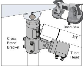
Fit Tube Head onto the MT to ensure proper fit, adjusting or modifying the MT as needed. Once verified, fully secure all fasteners.
