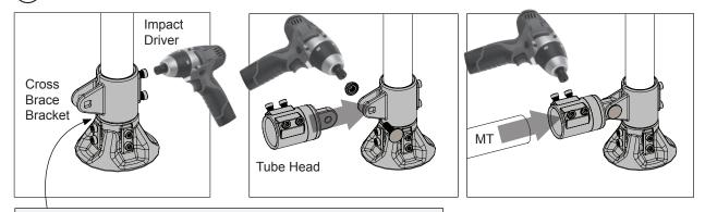
First Cross Brace Bracket should touch top of Base Foot.
