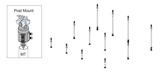
(C) WITHOUT FULLY SECURING THE BRACKET CLAMPS, install Rails onto the South row of Post Mounts.
