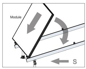
Before completely lowering the module, engage two Cam Feet at the back side of the module where they will meet their respective Rails. Fully rock the module down.
