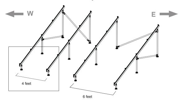
B Set a module onto the Tongue side of the Cam Foot Rockits. Align the module with the marked corner edge.
