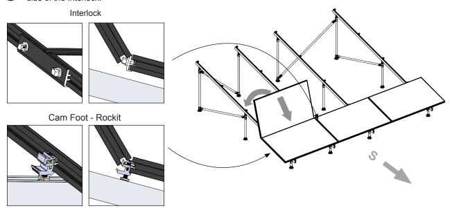
Before completely lowering the module, engage Cam Foot(s) at the back of the module where it will meet its respective Rail. Fully secure the Cam Foot(s).
