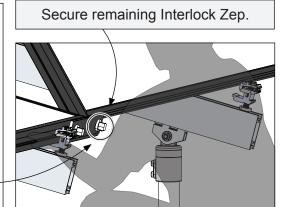
Before completely lowering the module, engage ONE Cam Foot at the back of the module where it will meet its Rail. Fully rock down the module and secure the Cam Foot with the Offset Flat Tool.
