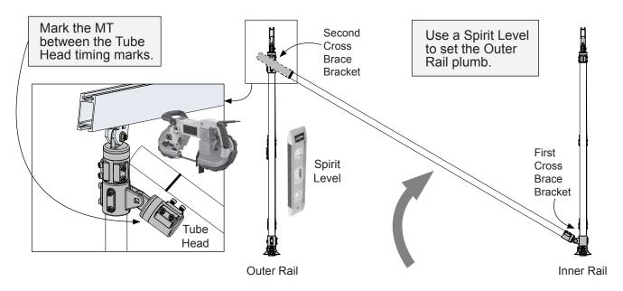
Fit Tube Head onto the MT to ensure proper fit, adjusting or modifying the MT as needed. Once verified, fully secure all fasteners.
