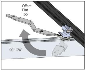
Install an Interlock Key-side in on the back of the two modules.
