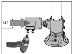
First Cross Brace Bracket should touch top of Base Foot.
