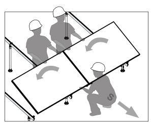
Install one Cam Foot onto the backs of the two modules where they will meet their respective Rails. Fully rock down the two modules and secure the Cam Feet with the Offset Flat Tool.
