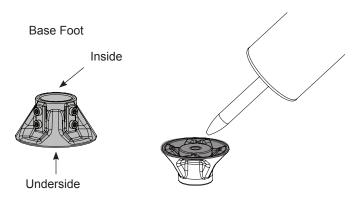
Place the Base Feet at the marked locations and secure in place with a Lag Bolt. Cover the inside of the Base Feet with 1/2" bead of sealant.
