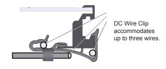
The example above shows pre-wiring or staging of modules prior to installation using the DC Wire Clip.
