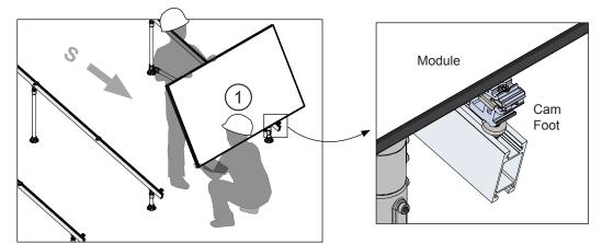
Have a third installer lift up a second module onto its Cam Foot while the second installer provides support.
